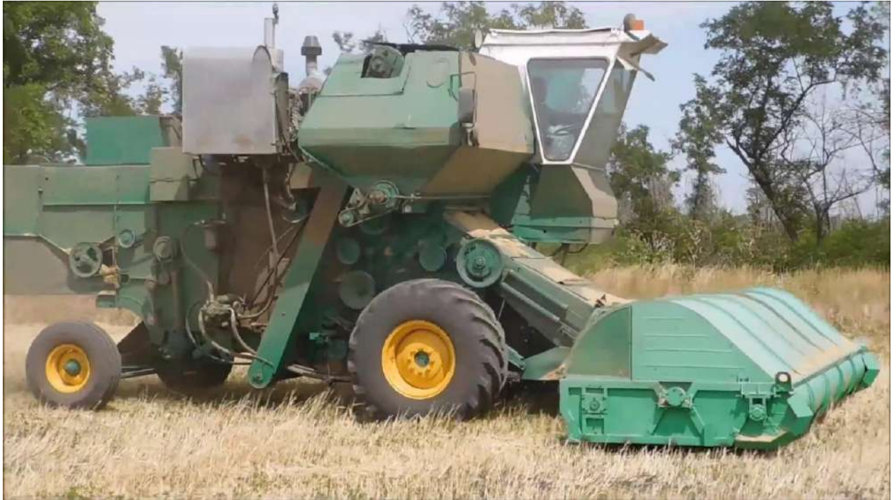
Figure 1.12 Combing header on the SK-5 "Niva" harvester
